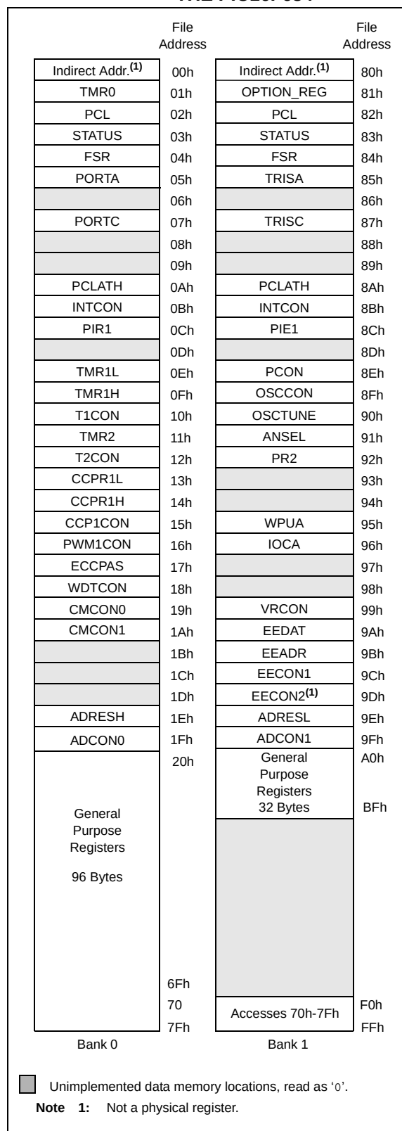
FIGURE 2-2: DATA MEMORY MAP OF THE PIC16F684
