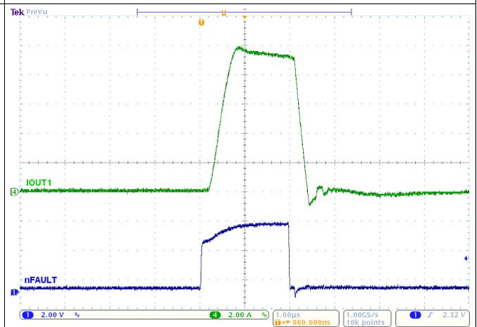
Figure 13. OCP With 24 V and Outputs Shorted Together
