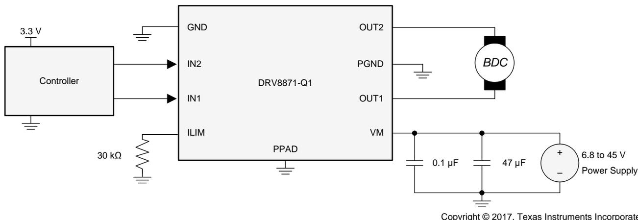
Figure 7. Typical Connections
